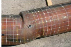
b) Observed Deformations of Steel Tube
